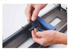
The splines on all the fixture plates can be reversed to accommodate parts using the inside diameter (ID) or outside diameter (OD). To reverse the spline orientation, pull the spring-loaded splines away from the plate and rotate them 180 degrees.
