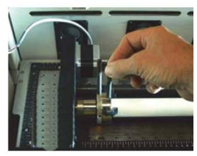
Cylinders can be held from the outside diameter or the inside diameter.
