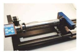
This photo shows a typical example of a larger part that requires a fixture plate on both the left and the right sides. Notice that the left side fixture plate is held in place with the 3-law Chuck
