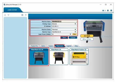
2. Your new laser has been activated in the Job Manager and now appears in the left panel. It is now ready to accept jobs from the print driver. Use the **Add or Delete** buttons to add or remove additional machines. Below you can see we have installed an additional FiberMark S2 laser system.
