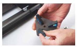
This photo shows the small idle-side plate fixture. The small plate fixture can accommodate sizes up to 1" in diameter.
